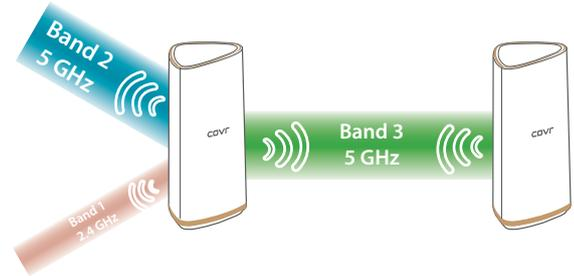
The Covr Tri Band Whole Home Wi-Fi System has a third separate band just for backhaul, leaving the other two bands unrestricted for connecting to your devices.
